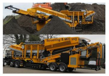
The starscreen can also screen cohesive soil in particular with a high throughput. The coarse fractions fall off in front of the machine. Mediumand finegrain fall to the rear and sides.
