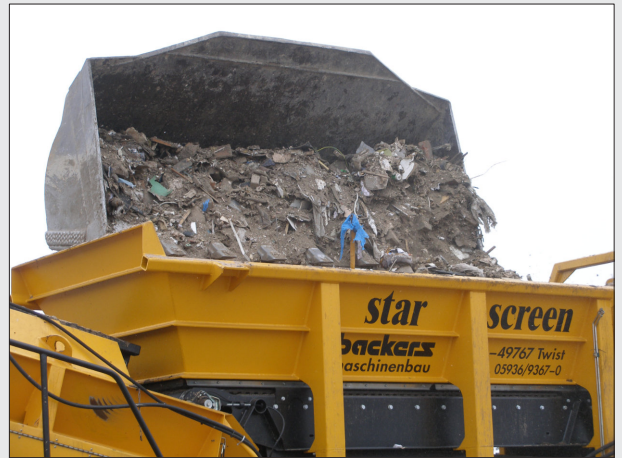
Excavator feeding of the 3-Fraction Starscreen 3-mtb
